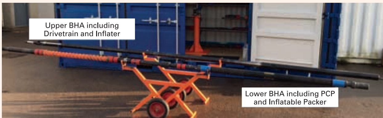
Fig. 12 Photo of the WIST BHA with an inflatable packer — Mk1 prototype.
