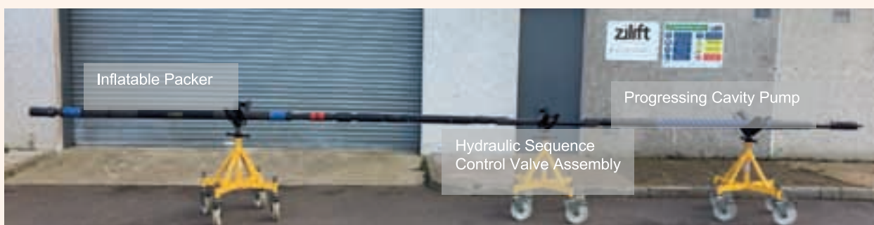
Fig. 13 Photo of the WIST BHA with an inflatable packer — Mk5 prototype.
