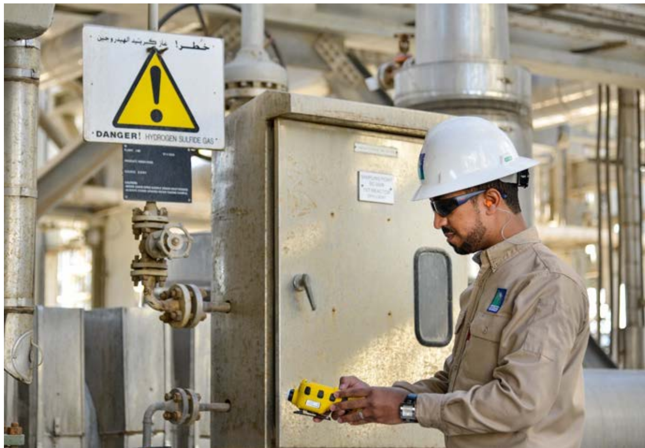
Figure 11: Utilization of direct measurement instrumentation to measure hydrocarbon occupational exposure at a facility by Lead Industrial Hygienist Ibrahim A. Al-Jabr, Saudi Aramco
